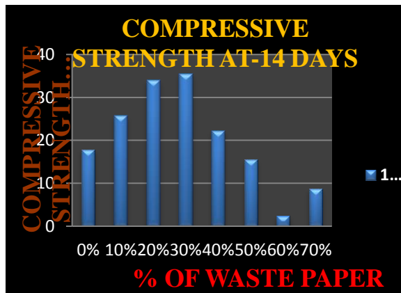
Fig. 2. Compressive Strength of Concrete Specimen at 14 – Days
